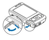
2 Insert a compatible memory card in the slot. Make sure that the contact area on the card is facing up and towards the slot.
