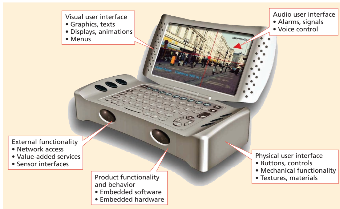
Figure 1. Virtual reality prototyping. VRP can use virtual and physical models in combination to provide the most effective simulation of the prototyped product's features. (CyPhone model courtesy of JP Metsävainio Design Oy, Finland.)
