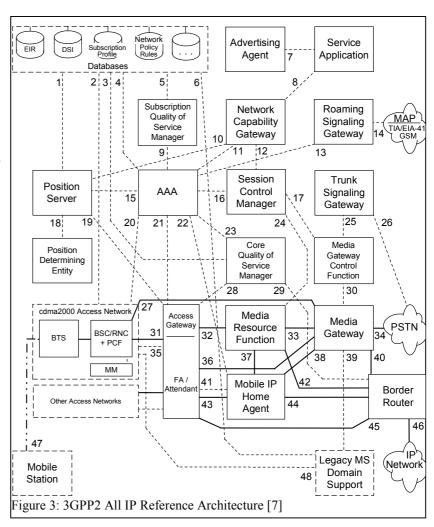
The Gateways of the 3GPP2 resemble very much the Gateways of the 3GPP. Media Gateway Control Function, Media Gateway, and Trunk Signalling Gateway of 3GPP2 have similar functionalities than MGCF, MGW, and T-SGW of 3GPP respectively. However, 3GPP2 introduces also Network Capability Gateway (NCGW), which main task is to authorise servers' use of the network resources. In 3GPP architecture functionality of NCGW is embedded into CSCF.
