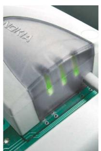
built in SIM card reader, internal antenna and interfaces for connecting to a remote device. This makes it an ideal communications link for a wide range of M2M applications, such as remote control and maintenance of utility meters, vending machines and industrial machinery, as well as telemedicine, security and surveillance devices. It can also be used as a normal wireless modem for connecting to the Internet.
