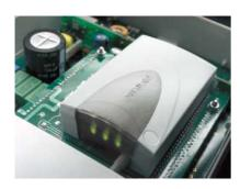
The Nokia 30 allows easy integration into machines and devices.
