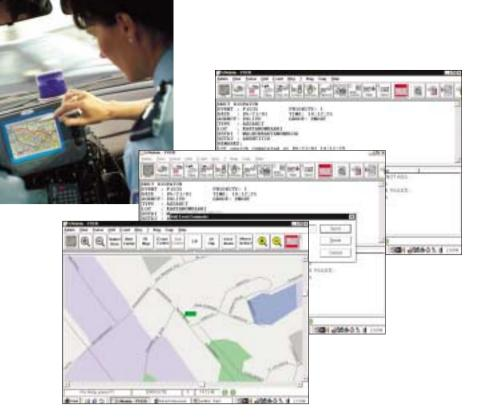
Vehicle locations are shown automatically on the map. Vehicles are fitted with a GPS based Automatic Vehicle Location (AVL) system, which uses TETRA SDS for communicating with the CAD system.
