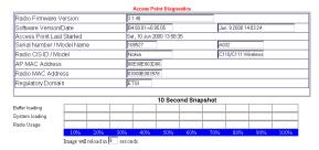
The first part of the screen provides information about the A032 and the PCMCIA radio cards (if inserted). The fields are explained below:
