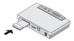
2 Take care to ensure that the card is aligned correctly and pressed all the way into the slot.
