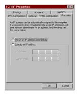
2 If necessary, delete any entries under the Gateway and DNS Configuration tabs (although DNS should still be enabled).
