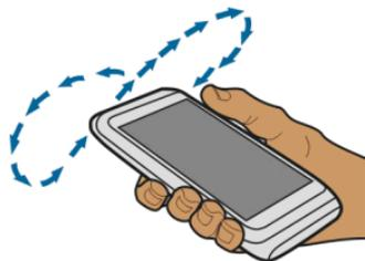
The compass has limited accuracy. Electromagnetic fields, metal objects, or other external circumstances may also affect the accuracy of the compass. The compass should always be properly calibrated.
