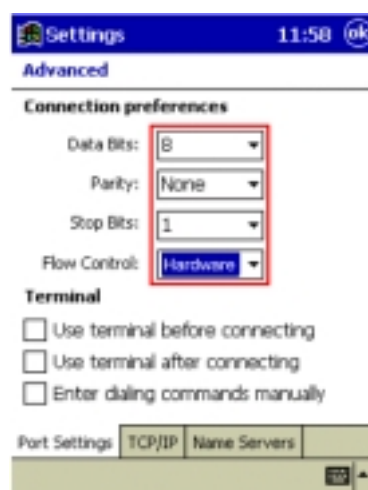
Figure 2. Check Connection preferences. Especially that the Flow Control selected is HW. Tap OK on upper right corner and then tap Next
