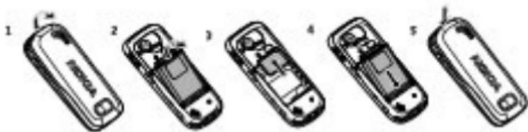
1. Press the release button and remove the back cover (1) and the battery (2).
