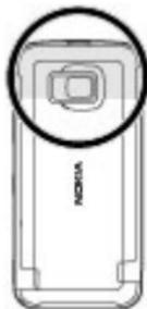
Antenne cellulare, Bluetooth e WLAN
