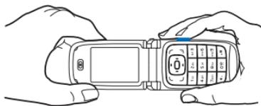
To zoom in and out in the camera mode, scroll up and down, or press the volume keys.
