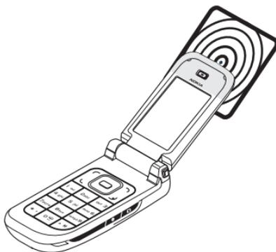
The reading range is typically 0 to 3 centimeters.
