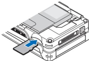
Use only compatible microSD cards with this device. Other memory cards, such as Reduced Size MultiMedia cards, do not fit in the microSD card slot and are not compatible with this device. Using an incompatible memory card may damage
