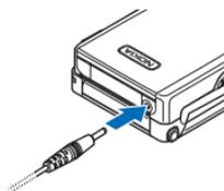
The charging time depends on the charger used. Charging a BL-4C battery with the AC-3 charger takes approximately 2 hours and 20 minutes while the phone is in the standby mode.
