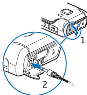
Do not connect products that create an output signal as this may cause damage to the device. Do not connect any voltage source to the Nokia AV connector.
