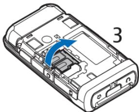
4. Insert the (U)SIM card to the SIM card holder. Make sure that the (U)SIM card is properly inserted and that the gold-colored contact area on the card is facing downwards.
