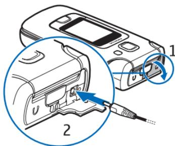
The charging time depends on the charger and the battery used. Charging a BL-5F battery with the AC-4 charger takes approximately 45 minutes.
