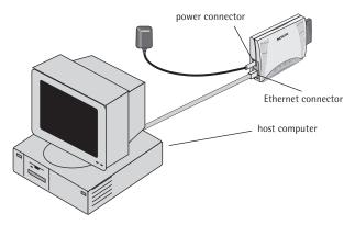
After the host computer has powered up, the adapter's **power** LED should glow a steady green, and its LAN LED should be on, indicating a good connection to the host computer.
