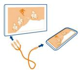
Do not connect products that create an output signal, as this may damage the device. Do not connect any voltage source to the Nokia AV connector. If you connect an
