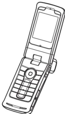
The Fold open mode is activated even if the fold is not fully opened. The fold opens close to 150 degrees, as shown in the picture. Do not force the fold to open more.
