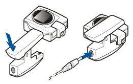
While charging, the screensaver is shown on the display. If Nokia Medallion II is switched on, after approx. 30 seconds it automatically switches the power off for more efficient charging.
