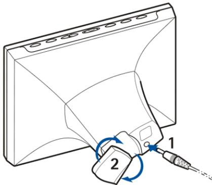
You can turn the table support (2) at the back to change the angle of the Nokia Image Frame display.
