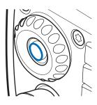
In direct mode, the group selector is used for selecting channels. The name of the channel is shown on the display. Each channel may have up to three groups. Pressing and holding the back key selects the first group (A) on the channel, and pressing the back key switches between the second and the third group (B and C) on the channel.
