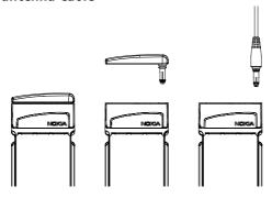
You can improve the reception and operating range of your Nokia Card Phone by using the External Antenna Cable XRP-2. It can be connected to any standard dual-band antenna that has a standard FME antenna connector.
