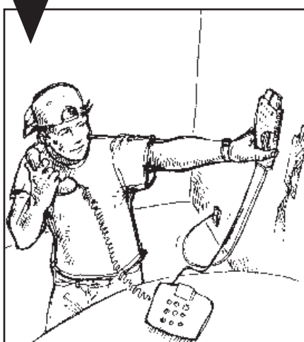
9. Check the GSM-field strength, if the test was not successful. Pick up the receiver and dial 777#. Move the terminal and observe the LED lights. Hold the terminal in an upright position.
