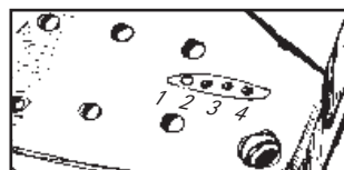
7. LED light 1 is first blinking and then continuously ON.
