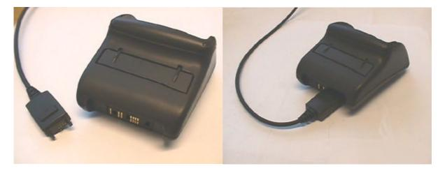
The button will not work unless Performance Travel Charger ACP-9 (supplied with Nokia 9110 Communicator or available as an accessory) is connected and *powered on*.
