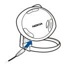
3. Disconnect the charger from the headset and wall outlet.
