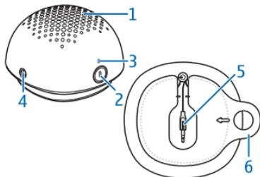
The speaker contains the following parts: speaker element (1), power key (2), indicator light (3), 3.5 mm audio connector (4), speaker cable with an audio plug (5), battery lid and coil for the cable (6).
