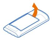
3 To unlock the memory card holder, slide it in the direction indicated by the arrow on the holder. Lift the holder.
