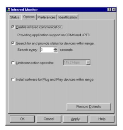
You can then check the infrared connection from the Status page. Activate your mobile phone's infrared transfer from the Infrared menu and make sure that the infrared ports of the two devices are pointing at each other. If the connection works, the text *One available infrared device is within range* should appear in the Infrared Monitor window.
